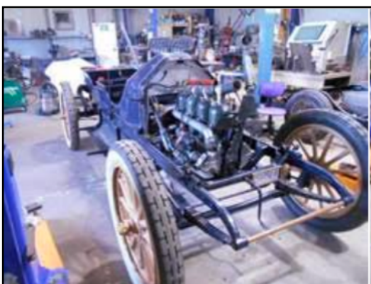
Body removed for further inspection work on mechanical parts
