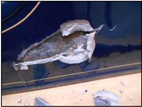
More plastic Bondo than metal - no wonder it had developed paint cracking
