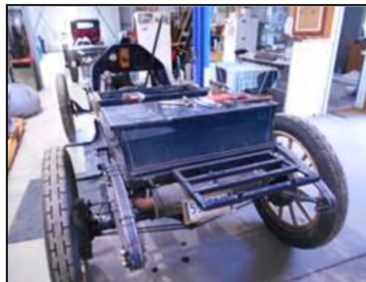
Body removed for further inspection work on mechanical parts
