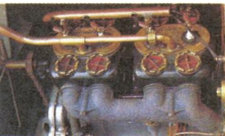
The bi-block T-head engine is set well back in the chassis
