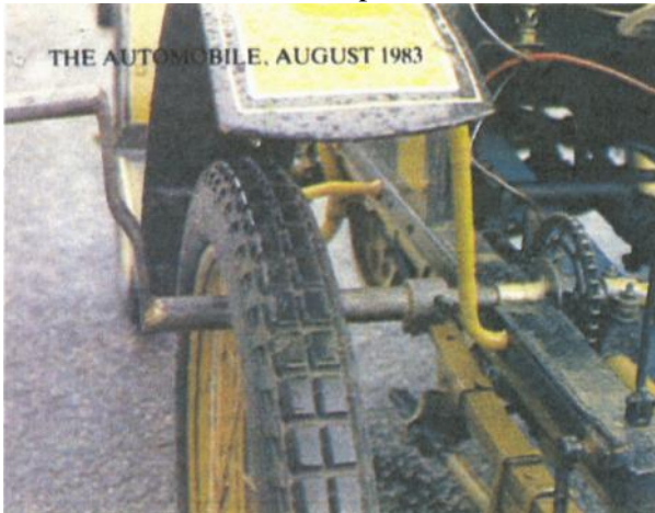
Prior to the invention of electric starting transversely mounted engines always presented the problem of arranging access for the starting handle - on the 1901 Pick the handle passes through the spokes of the front wheel.
