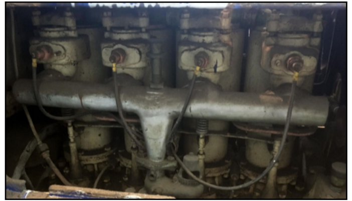
The Panhard engine in its current form, fitted with a Schebler carburettor
